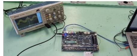
Fig. 8. Test setup, consisting of the oscilloscope, laptop, FPGA, and RC load
